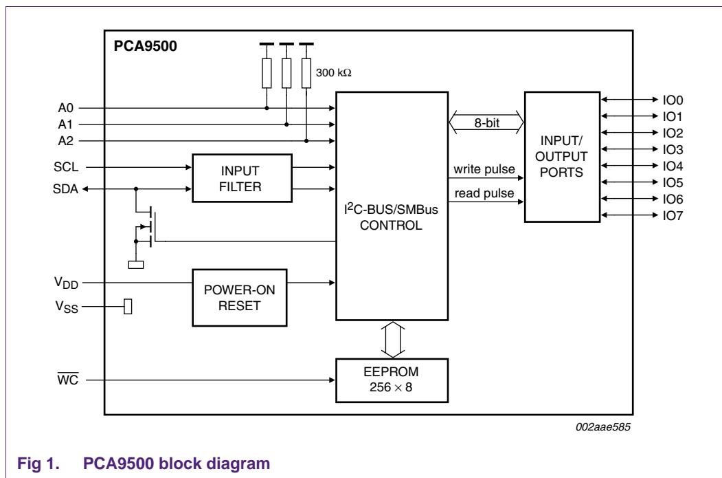
Fig 1. PCA9500 block diagram
