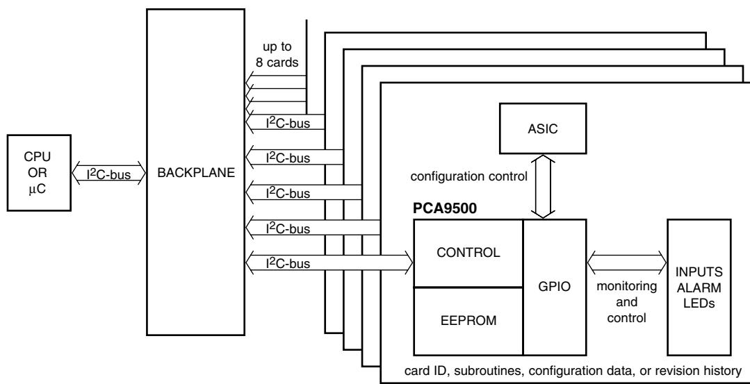
Fig 3. System level utilization of PCA9500
