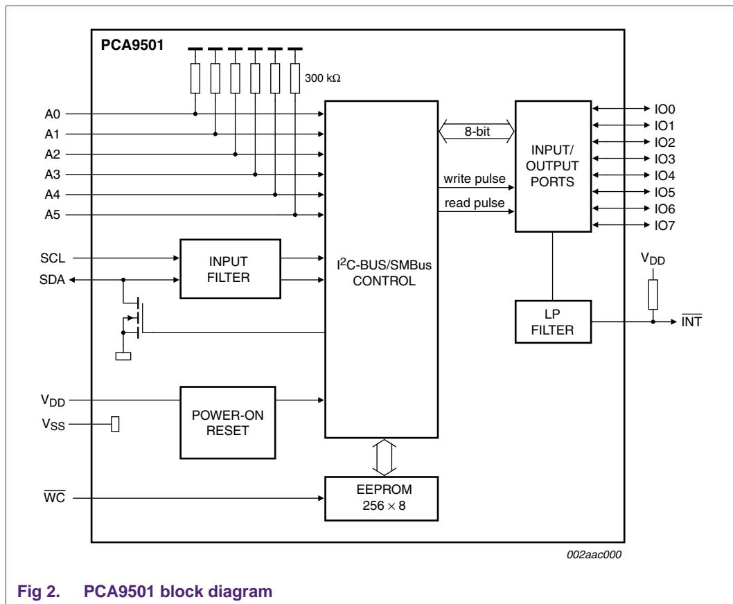
Fig 2. PCA9501 block diagram
